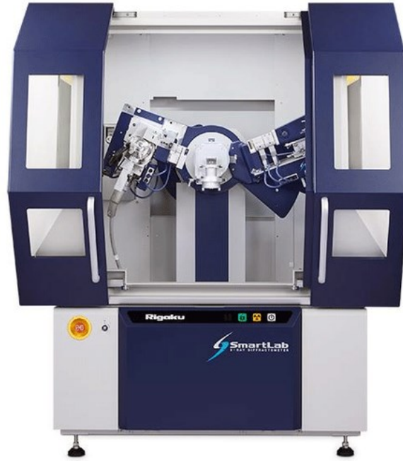
Figure 4-1 Rigaku Smartlab XE diffractometer of the Chemistry Department of University of Parma.
