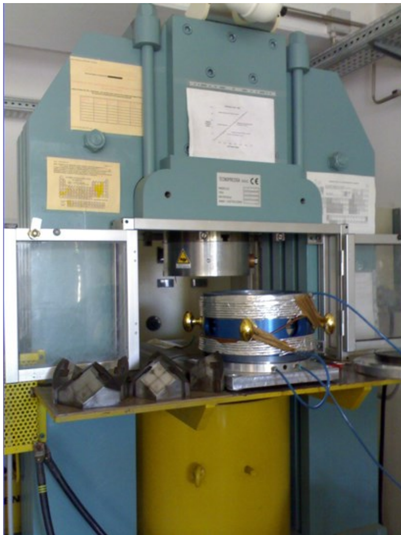
Figure 3-2 Walker-type multi-anvil press at IMEM-CNR (Parma, Italy).
