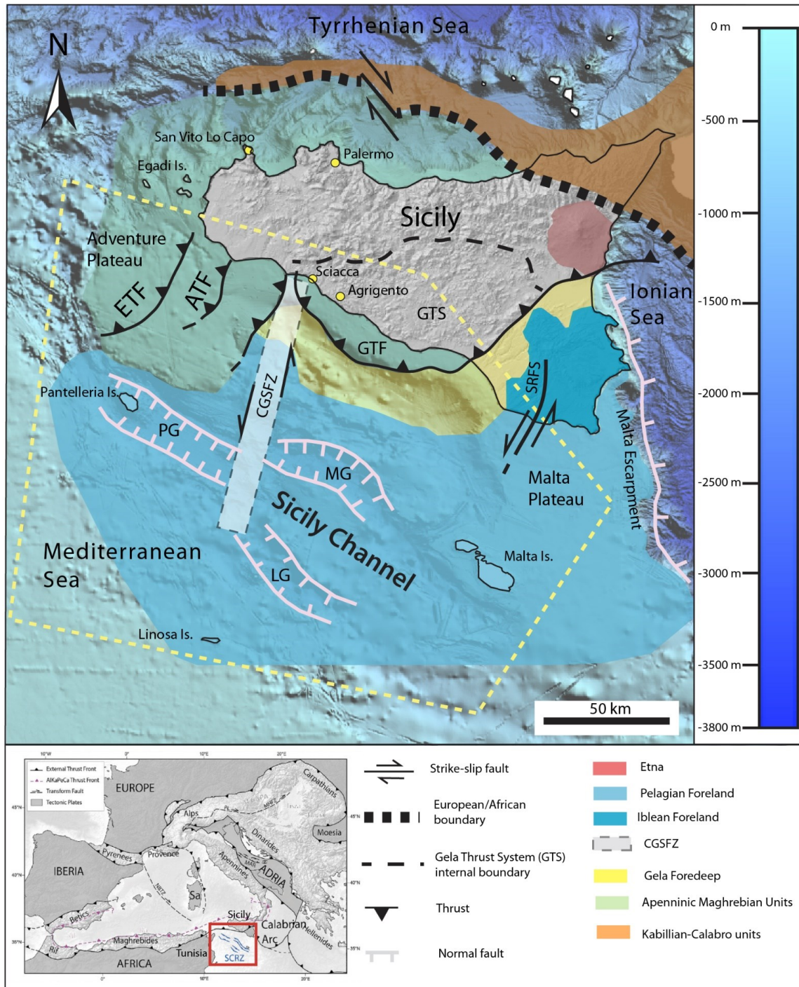
Fig. 3.1. Bathymetric map showing the main structural elements of the Sicily Channel region - AP: Adventure Plateau; ATF: Adventure Thrust Front; CGSFZ: Capo-Granitola Sciacca Fault Zone; SRFS: Scicli-Ragusa Fault System; ETF: Egadi Thrust Front; GTF: Gela Thrust Front; GTS: Gela Thrust System; MG: Malta Graben; LG: Linosa Graben; PG: Pantelleria Graben (after Maiorana et al., 2024, in: Gasparo Morticelli et al., 2015; Civile et al., 2018; Sulli et al., 2021). The localization
