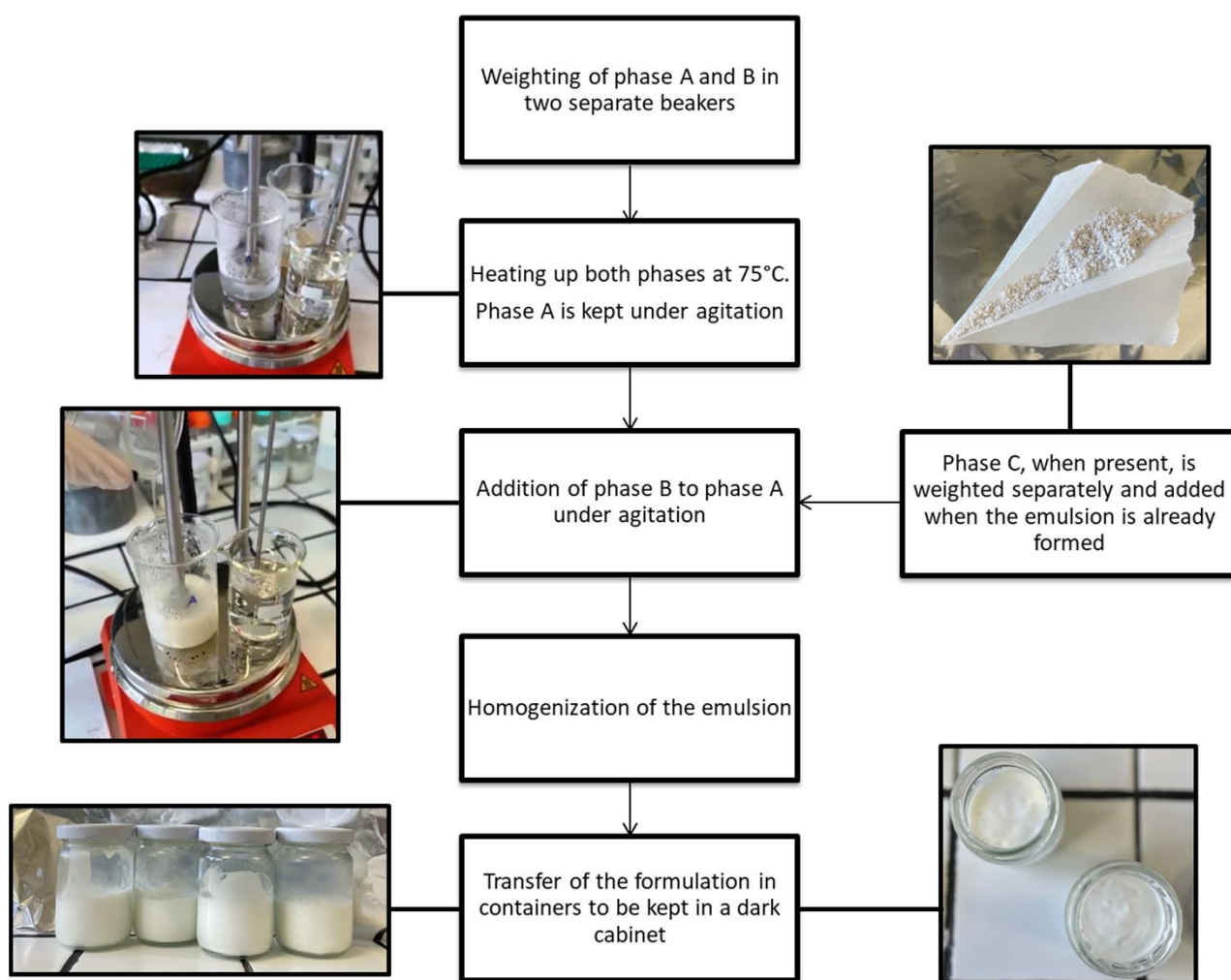
Figure 213. A schematic representation of the emulsion preparation process
