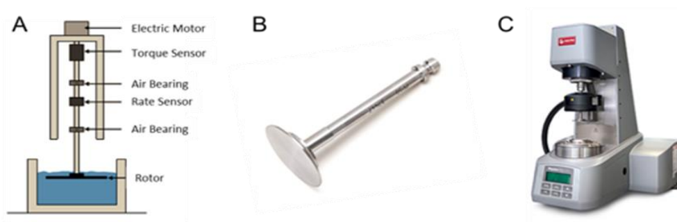
Figure 111 A) Scheme of the hydrodynamic resistance measurement set-up B) Aluminum alloy Rheometer Disk D-PP50/AL/S07D by Anton Paar used as substrates C) Anton Paar Rheometer MCR 301.
