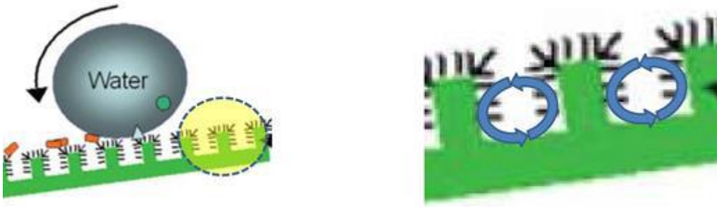
Figure 103 Principle of operation of a superhydrophobic coating, illustrated in the case of a drop of water rolling along an inclined plane coated with superhydrophobic surfaces.
