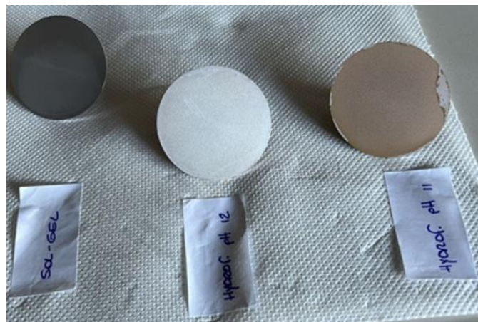
Figure 121 Comparison of the hydrodynamic resistance results of the smooth aluminium disc used as reference and of the coated surfaces: “Sol-gel”, “pH12 Urea”, and “pH11 No Urea”, before the liquid infusion.
