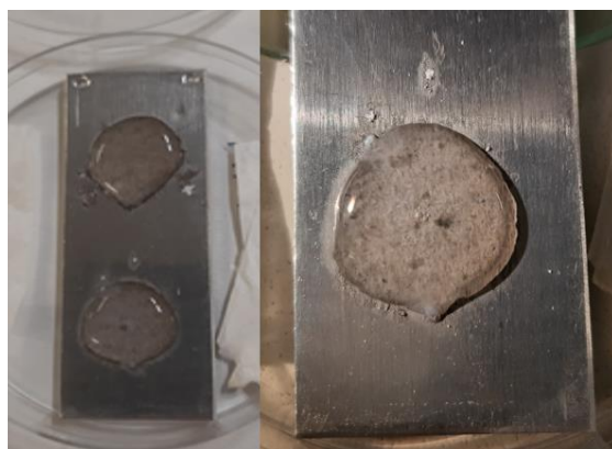
Figure 73 Smooth aluminum substrate at the end of “droplet assay”. Substrate corrosion and the development of aluminum oxides and hydroxide are observed.
