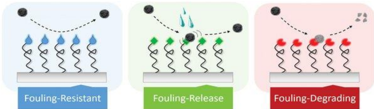
Figure 5 Schematic illustration of three principal antifouling strategies 1) fouling resistant, 2) fouling release and 3) fouling degrading 30 .
