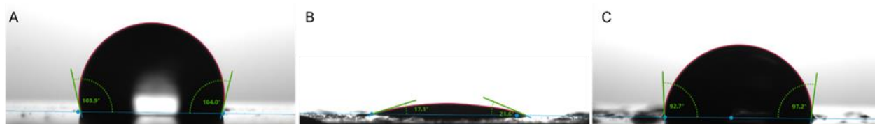
Figure 120 Sessile contact angle of water of the SLIPS surfaces used as candidate for hydrodynamic resistance test: A) “Sol-gel” + Vaseline ,B) “pH12 Urea” + Vaseline, C) “pH11 No Urea” + Vaseline.
