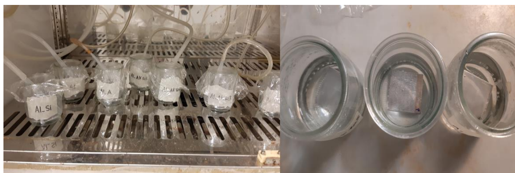
Figure 75 Collection of leaching products of aluminum specimens (3x3 cm) covered by the experimental coatings.
