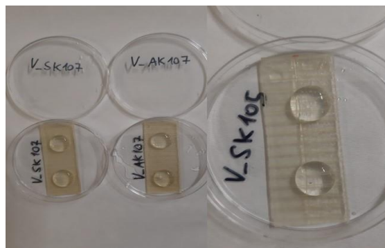
Figure 72 Example of “droplet test” on fiberglass substrate.
