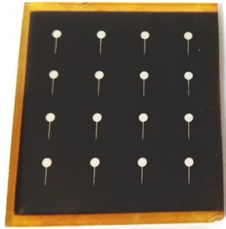
Figure 6.6 - Standard test sample, later mechanically scribed into 16 solar cells of area=0.05 cm 2 . The brownish frame is due to the CdS deposition: it was etched on one edge to realize the contact with the TCO at the back, by means of Ag paste.
