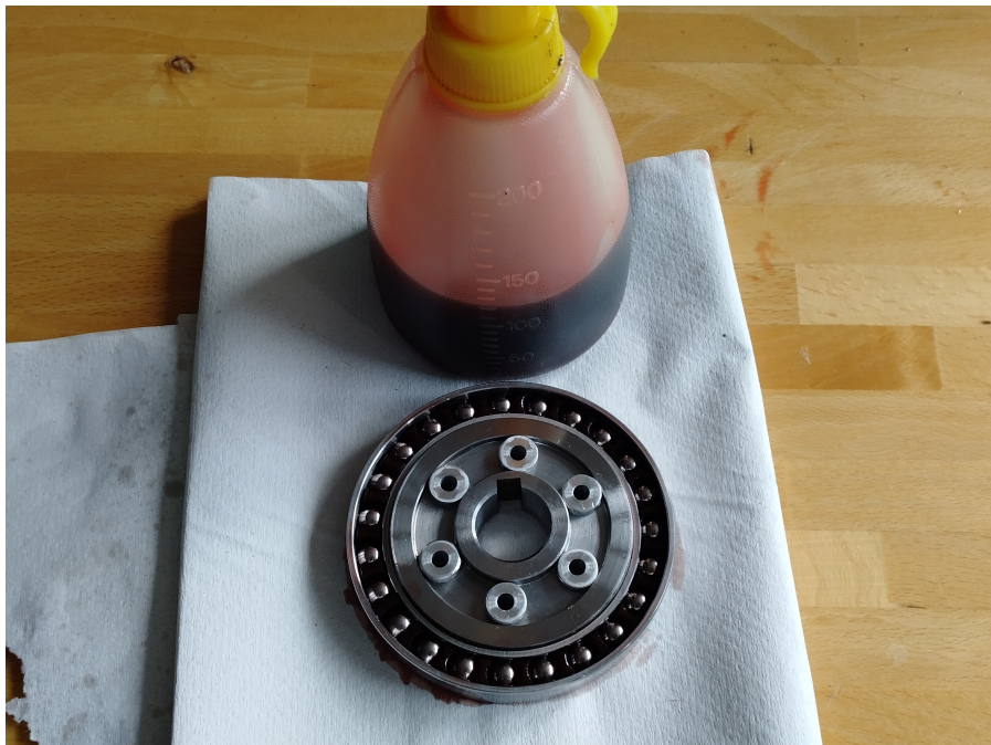
Figure 86: Lubrication of gearing wave generator.
