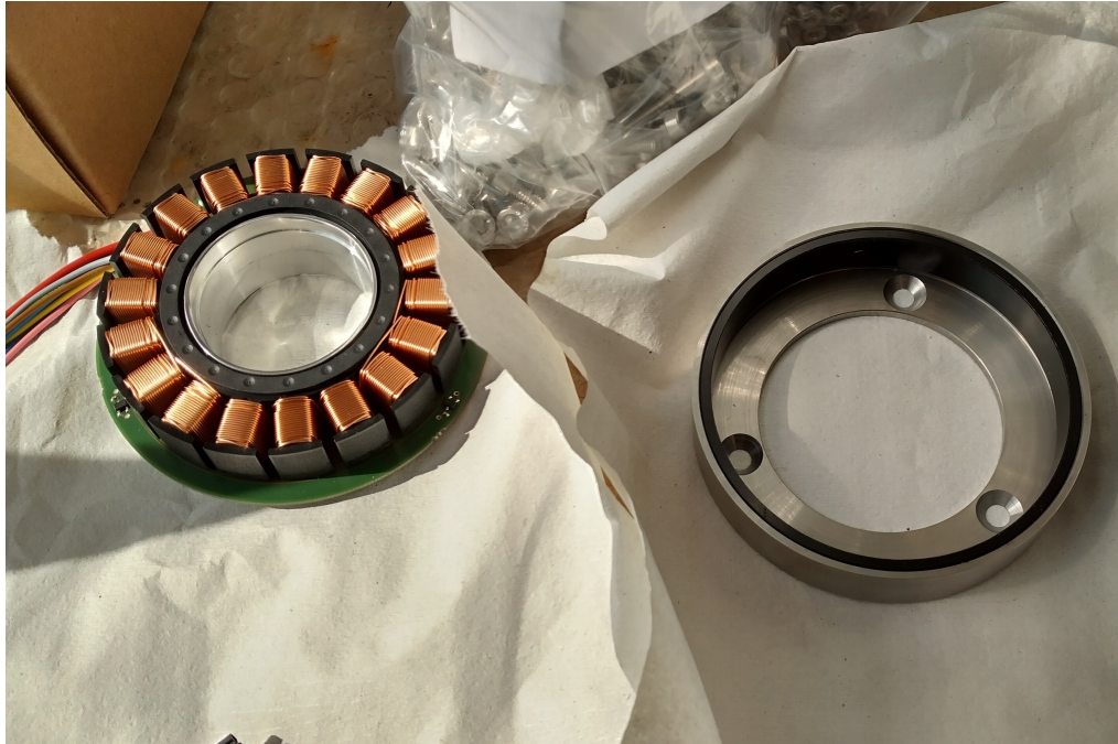
Figure 83: BLDC motor stator windings and magnetic rotor, characterized by hollow and significantly flat design.
