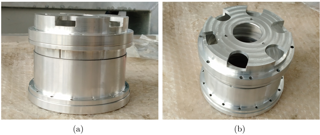
Figure 80: Complete drive casing, unscrewed: (a) side and (b) rear view.
