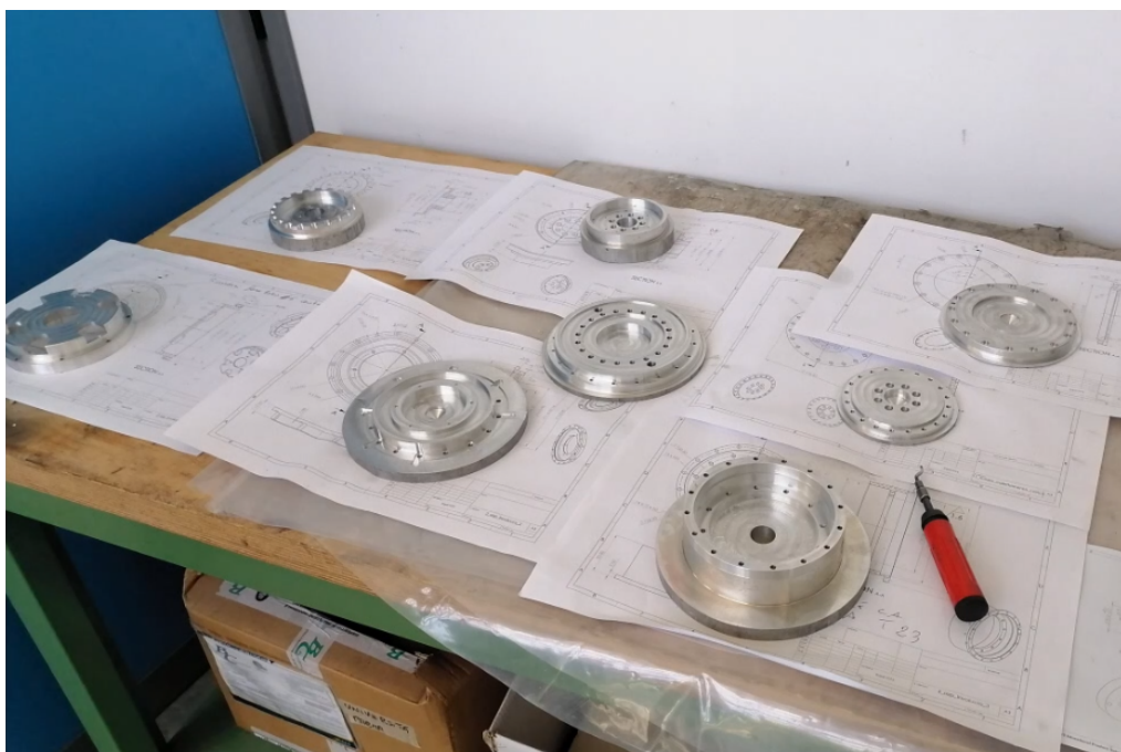
Figure 78: View of some manufactured parts, with respective drawings.
