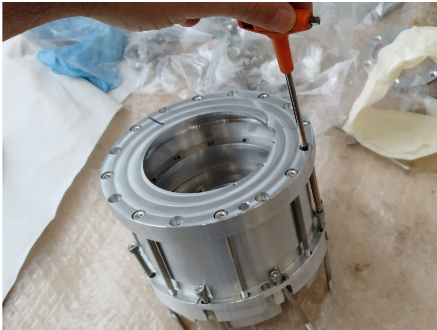
Figure 82: Detail of drive casing installation procedure. A common straight Allen wrench is used to quickly fasten/unfasten the drive to robot casing, without need for removable covers (see also Fig. 30a).
