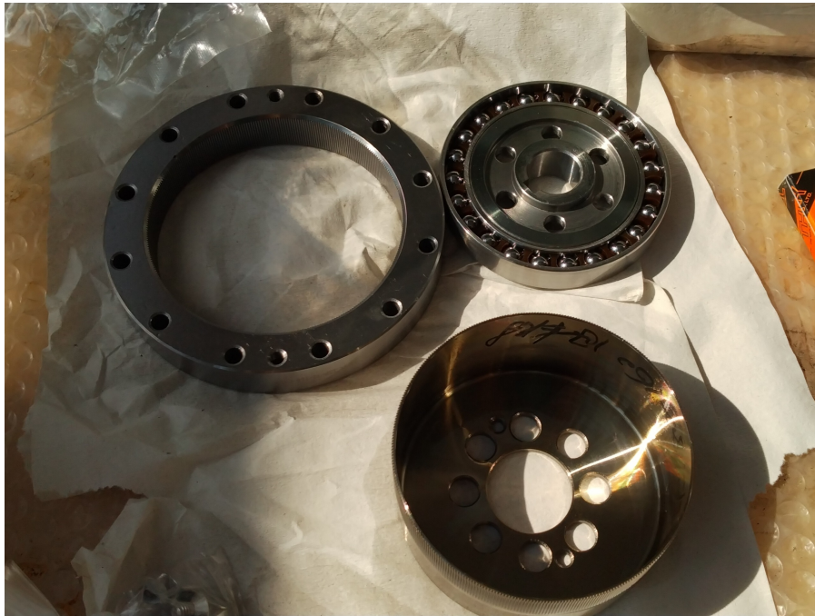
Figure 85: Harmonic drive gearing component set parts: wave generator, flex spline, circular spline.
