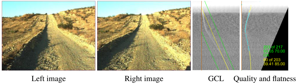
Figure A.4: V-Disparity image analysis in a non flat ground scene. Set A points are plotted in yellow and set B points in cyan.
