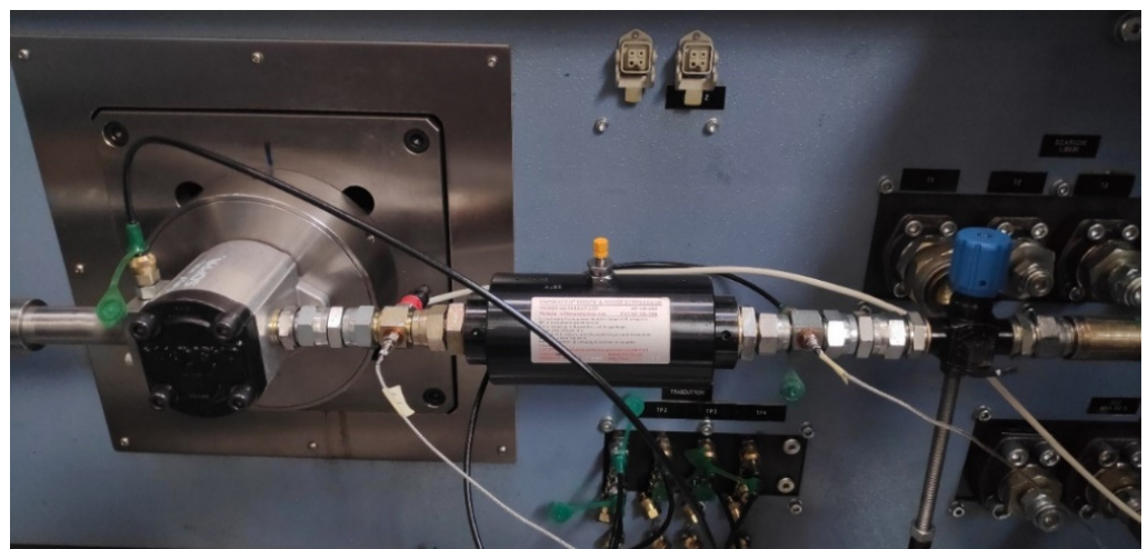
Figure 3. Pump and suppressor at the test bench.
