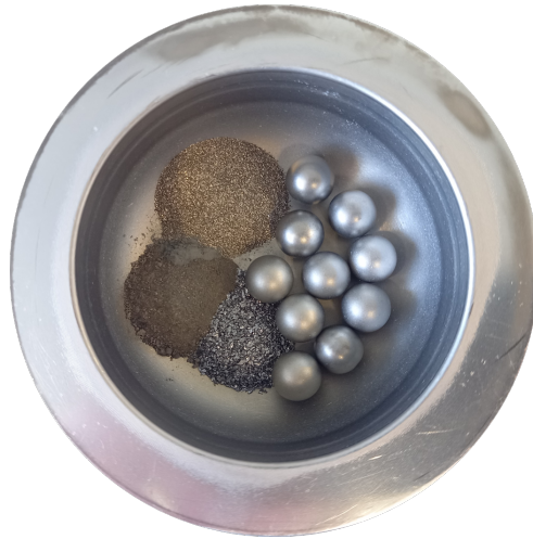
Figure 5.1: Steel jar for high energy ball milling containing precursor powders and milling balls before starting the milling process.
