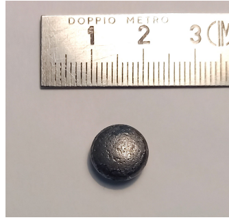
Figure 3.1: NiMnIn ingot obtained by arc melting.
