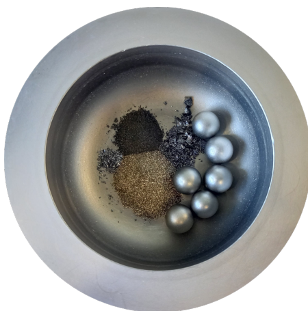
Figure 6.1: Steel jar for high energy ball milling containing precursor powders and milling balls before starting the milling process.
