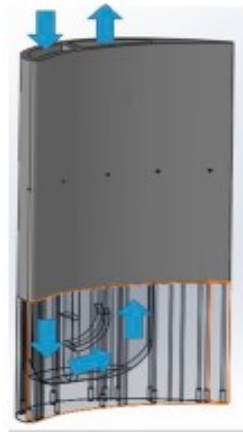
Figure 4.11 – Internal convective cooling channel [113]
