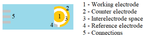
Figure 7.1. Schematic representation of the screen-printed electrode: working (1) and counter (2) gold electrodes, ceramic interelectrode space (3), silver reference electrode (4), electrode connections (5)
