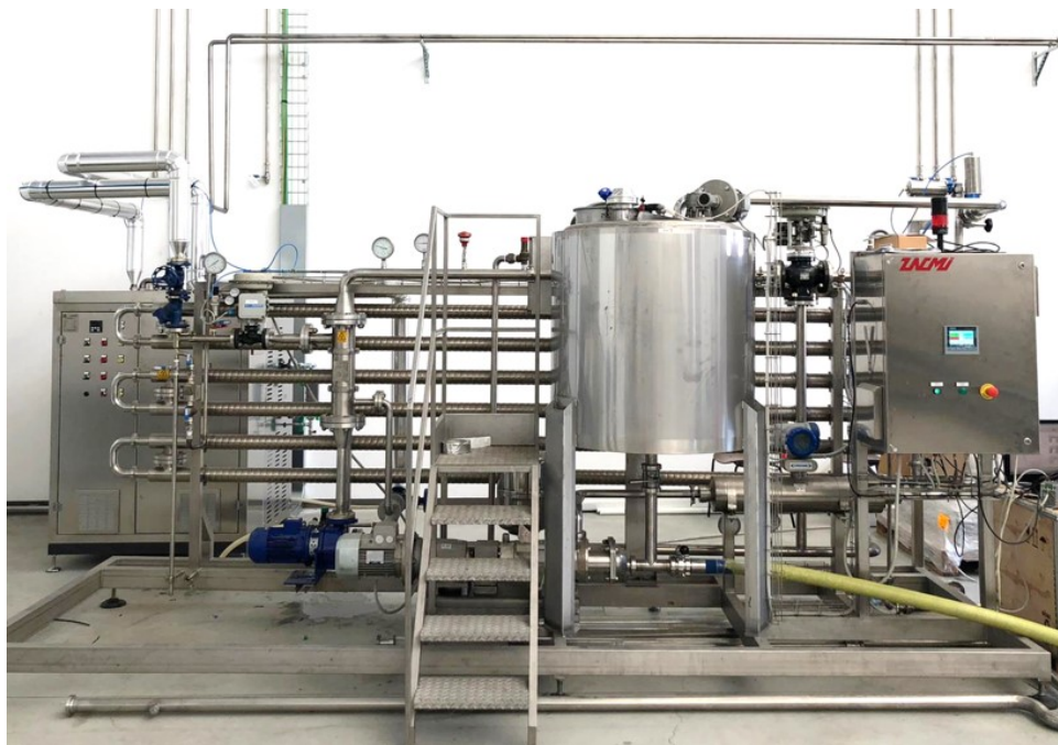
Figure 4.39: Pilot plant for the thermal treatment of viscous fluids installed at the University of Parma.
