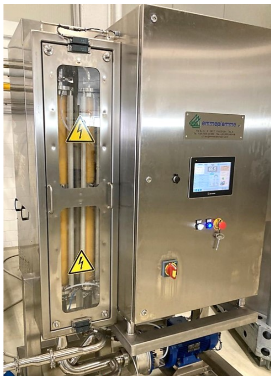
(a) Continuous industrial ohmic heater used with liquid egg products.
