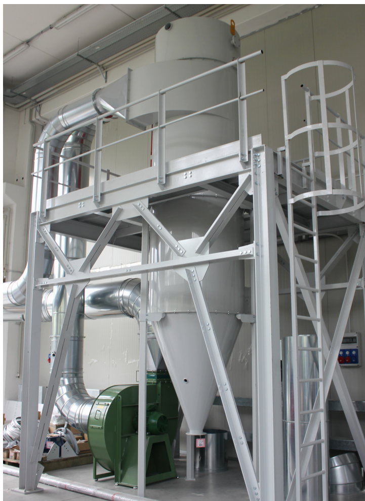
Figure 3.22: Cyclonic bag filter pilot plant used for experimental testing
