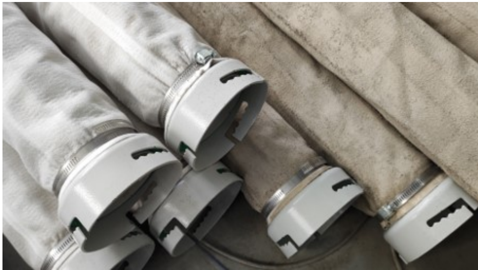
Figure 4.7: Comparison between clean (on the left) and completely clogged filtering bags (right) disposed of by an industrial manufacturer.
