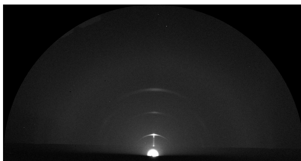
Figure 3.14 Example of CCD raw data XRD image collected at the synchrotron facility
