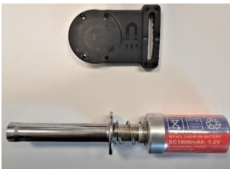
Figure 9 Strong magnet and battery for interference test
