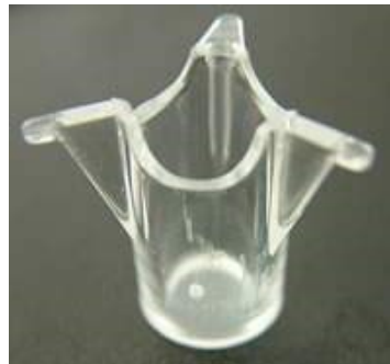
Figure 7 24-well plate cell culture insert. rCMs were cultured on the inserts, while MSCs were growing on the bottom of the well.
