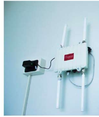
(b) Meshlium Xtreme Access Point to monitor indoor occupancy based on Wifi and bluetooth active devices.
