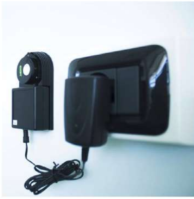
(a) Plug and play Fixed Sensor to monitor temperature, relative humidity and CO 2 concentration
