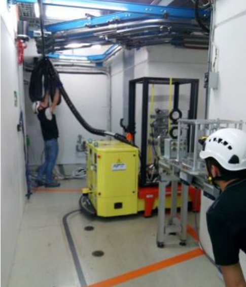
Fig. 4 – The automated conveyor chariot.
