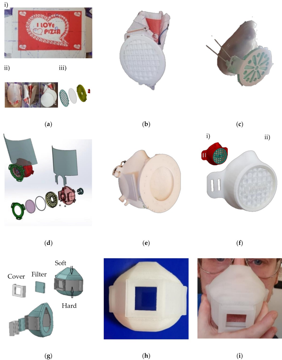
Figure 1. Prototyped masks: (a) Schematics of emergency masks, (i) shape design, (ii) details of mask, (iii) details of filter support; (b) Details of paper mask and 3D printed PLA filter support; (c) Filter support connected with a typical hospital silicone mask; (d) Schematics of eco-masks for hospital use; (e) Detail of hospital eco-mask with removable support filter; (f) eco-mask for industrial use with lock-grid for filter change: (i) model design, (ii) prototyped mask; (g) Schematics of self-adaptable masks fabricated with droplet-based precision extrusion deposition (db-PED); (h) Detail of resting mask shape; (i) Final shape of the universal self-adaptable mask, obtained with PED technology.
