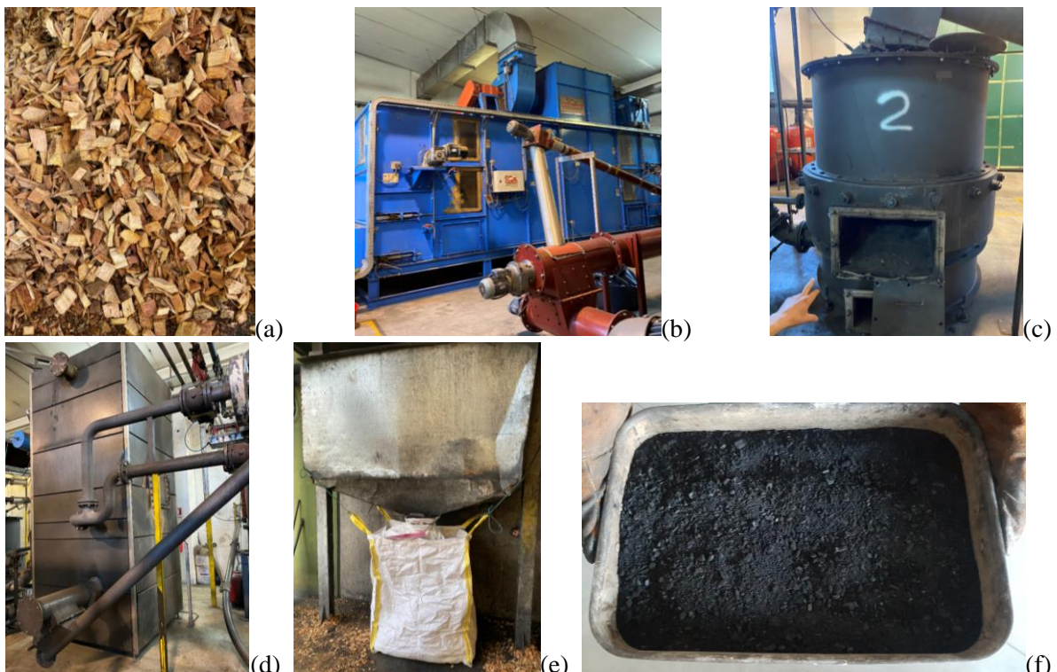
Figure 2 – (a) Input woodchip biomass; (b) drier; (c) gasifier; (d) component for syngas filtering and cooling; (e) biochar collection; (f) biochar used for the experimental campaign.
