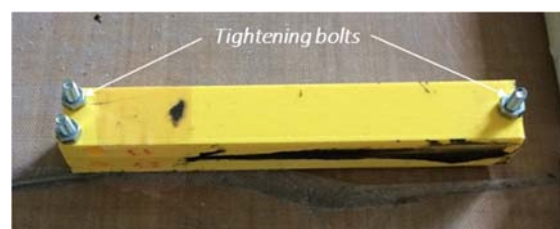
Figure 3. Bonding procedure: placing of spacers and polyester sheet (a); closing of the joint by tightening bolts (b).
