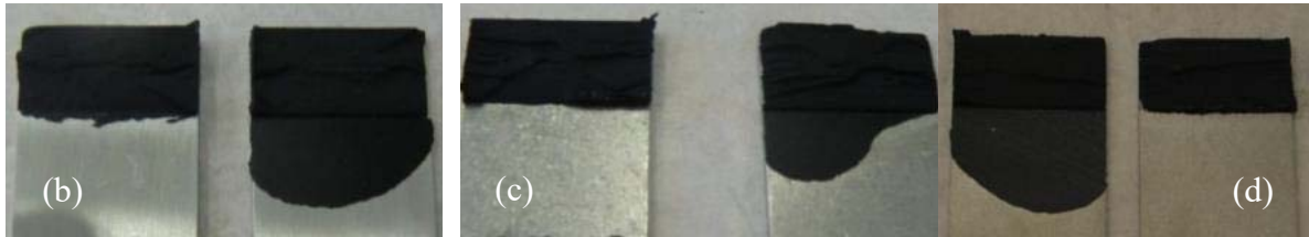
Figure 12 – Failure surfaces of the specimens made with Adhesive 3 and Scotch-Brite (b), 2B tumbled (c) and Shot-peened (d) surface finish.
