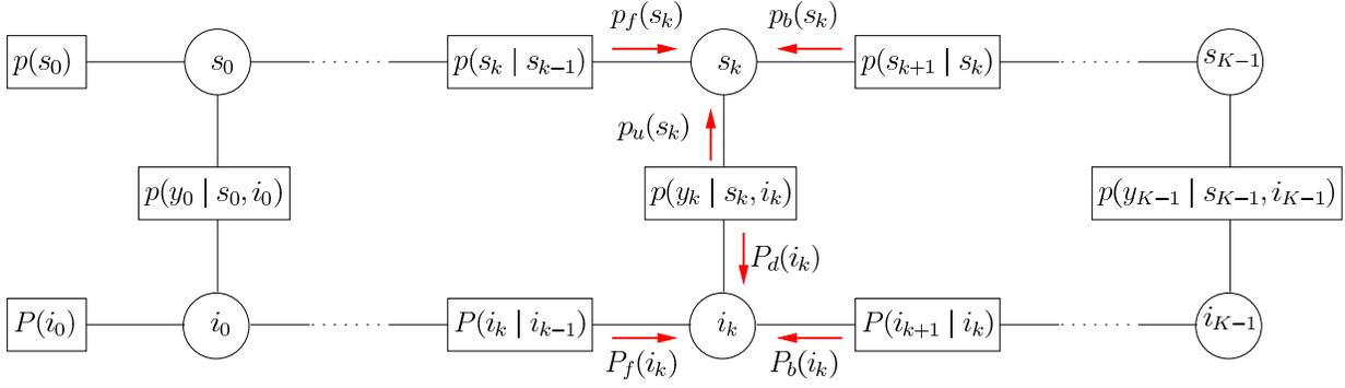
Figure 1. FG modelling the joint probability distribution function  $p(\mathbf{s}, \mathbf{i} | \mathbf{y})$ . The  $k$ -th stage is highlighted along with messages sent from factor nodes to variable nodes. The initial ( $k = 0$ ) stage is driven by the priors,  $P_f(i_0) = P(i_0)$  and  $p_f(s_0) = p(s_0)$ , while  $P_b(i_{K-1}) = p_b(s_{K-1}) = 1$  for the last ( $k = K - 1$ ) stage.
