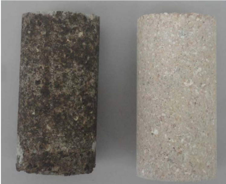
Figure 3: RAP-CBT specimen on the left, Virgin-CBT specimen on the right
