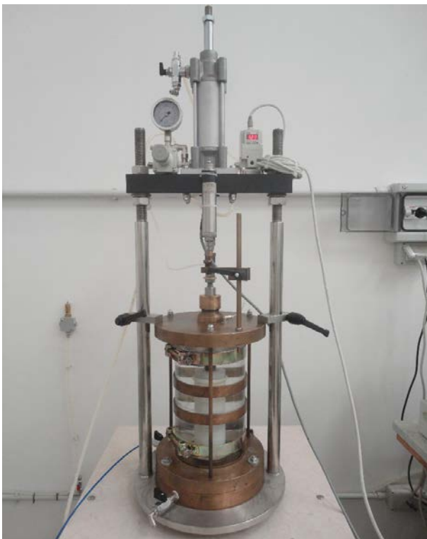
Figure 4: Cyclic Triaxial Test Configuration
