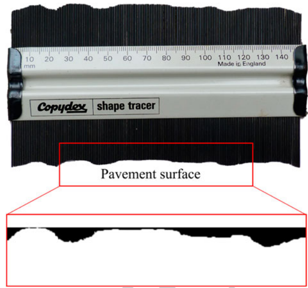
Figure 4. Pavement profile obtained from the Barton comb.
