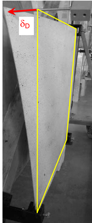
Fig. 7. Side view of the plate specimen, under prescribed displacement of 100 mm at corner D: the significant deflection can be appreciated.
