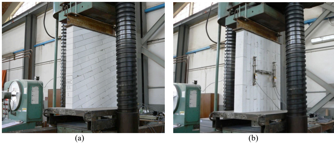
217 Figure 3. General setup of uniaxial compression tests performed under loading control: (a) not 218 instrumented and (b) instrumented small-scale masonry panels (PMC).
