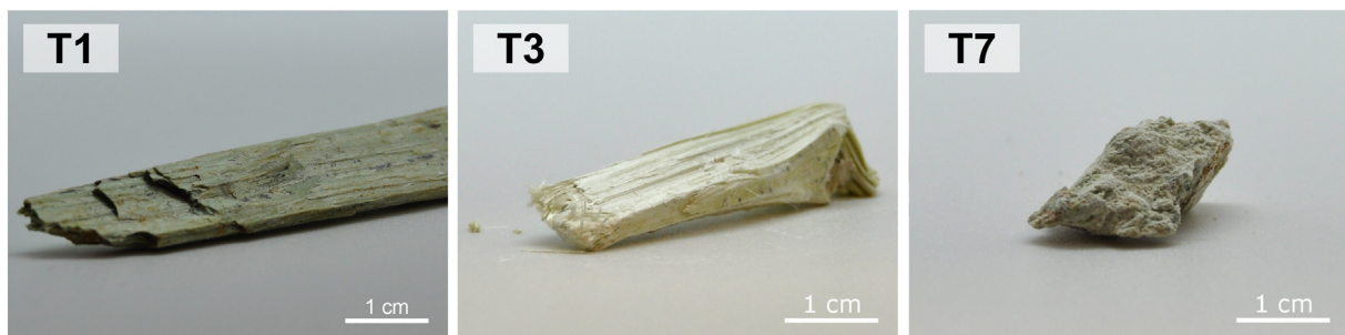
Fig. 4. Macroscopic description of the three cohesive state of antigorite specimen from nickel ores. The representative images describe the different cohesion of natural occurring antigorite samples, from massive to moderately to weakly cohesive (T1, T3, and T7, respectively).
