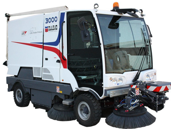
Figure 1. A typical three-brushes street sweeper (image courtesy of Dulevo International S.p.a.).
