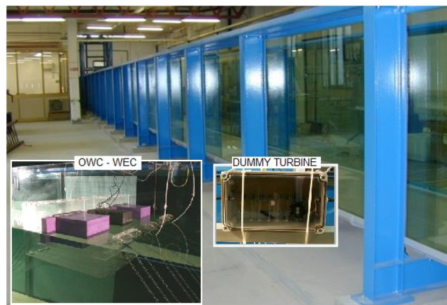
Figure 18. Wave flume of the Maritime Laboratory at the University of Padua.
