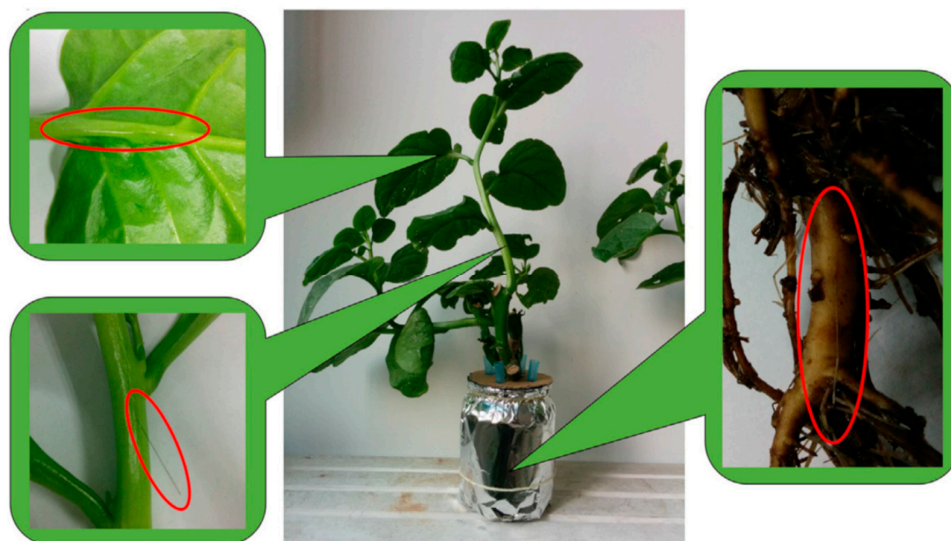
Figure 7. In vivo SPME sampling in different organs (leaf, stem and root) of living malabar spinach plant with custom-made PDMS fibers. Reprinted with permission from [78].
