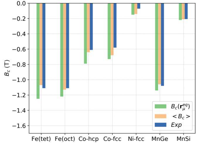
FIG. 3. Contact hyperfine field  $B_c(\mathbf{r}_\mu^{\text{eq}})$  at the equilibrium muon implantation position  $\mathbf{r}_\mu^{\text{eq}}$ , the muon contact field averaged over the muon wave-function spread,  $\langle B_c \rangle$ , and experimentally observed values.
