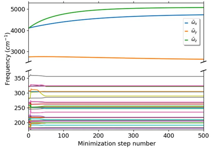
FIG. 4. Evolution of the SSCHA muon frequency ( $\tilde{\omega}$  in the upper panel) and those of Fe (nearly static low-frequency lines in the lower panel) during minimization for the muon in the tetrahedral site of bcc Fe. The figure depicts the expected anharmonicity effects on the SSCHA muon frequencies and nearly nonexistent anharmonicity effects on those of Fe, due to the large mass difference of the muon and Fe nuclei. The muon is  $\approx 490$  times lighter.
