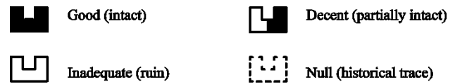
Figure 2. A proposal for the symbology regarding the state of conservation of fortified buildings
