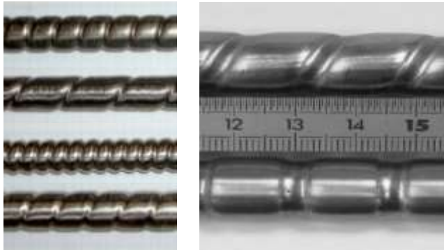
Figure 1. Representative spirally and transversely corrugated pipes.
