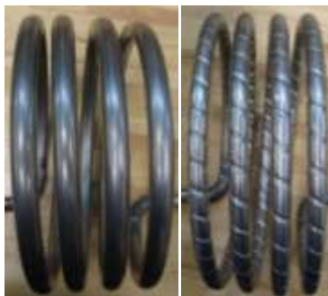
Figure 2. Representative smooth and corrugated helically coiled pipes.
