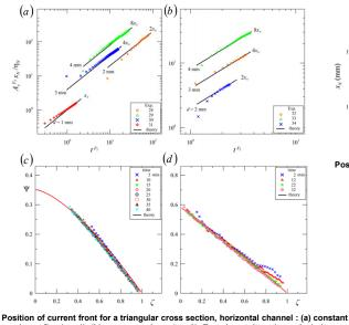
volume flux ( $\alpha = 1$ ); (b) constant volume ( $\alpha = 0$ ); Experimental vs. theoretical shape function at different times for: (c) test #34 ( $\alpha$  = 1); (d) test #29 ( $\alpha$  = 0)
