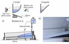
(a) Experimental setup; (b) Gravity current for  $\alpha=1$ ,  $\beta=1$ , n=0.75
