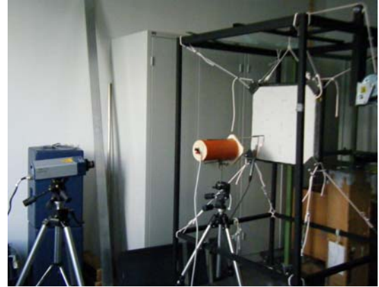
Figure 4. Experimental set-up of the LDV&microphone test.
