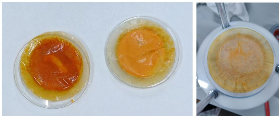
Figure 173 – Filtering cellulose-based capsules containing the adsorbent phase made of bentonite-hydrotalcites pellets after the adsorption of methyl orange. Wet and dried capsules.
