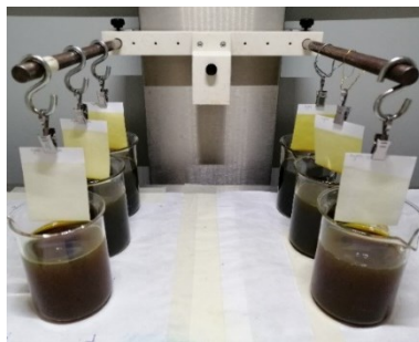
Figure 91 – Image representing the dip-coating deposition of AgNPs on paper substrates at different silver concentrations.
