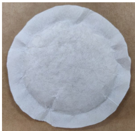
Figure 172 – Cellulose-based capsule containing bentonite-hydrotalcite Pural MG70 (weight ratio 70:30) grinded pellets.
