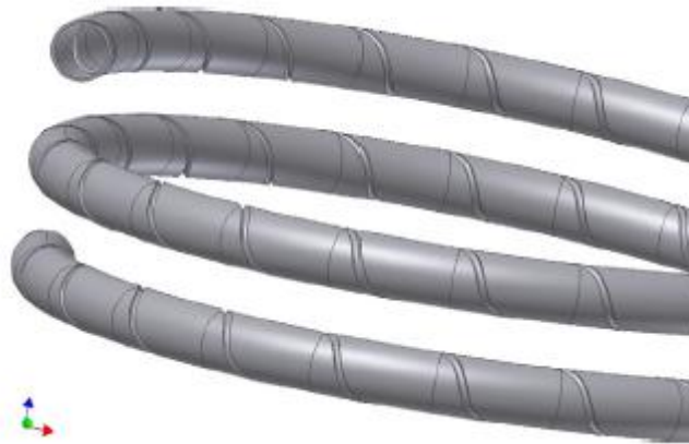
Figure 1.15: Schematic geometry of the corrugated coiled tube heat exchanger considered by Zachar (2010).
