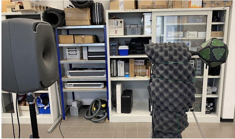
Figure 119. Measurement setup showing the loudspeaker and the DUT on the turntable.
