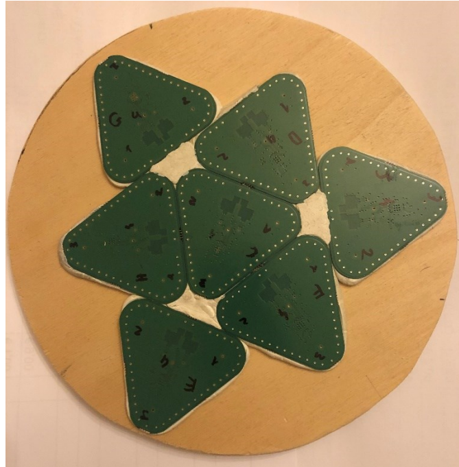
Figure 99. Prototype of the realized planar microphone array with 7 triangular arrays (28 capsules).
