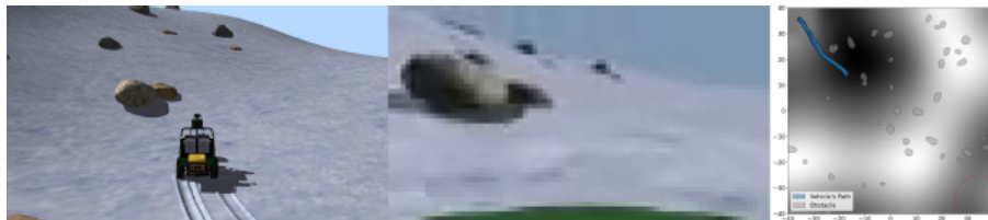
Fig. 4: Snapshot of a scenario used for testing. Left: third-person perspective of the vehicle; center: image from the camera’s view at the resolution used in training 80 \times 45 pixels; right: the current progress of the vehicle amount the hills and obstacles corresponding to the images on left.
