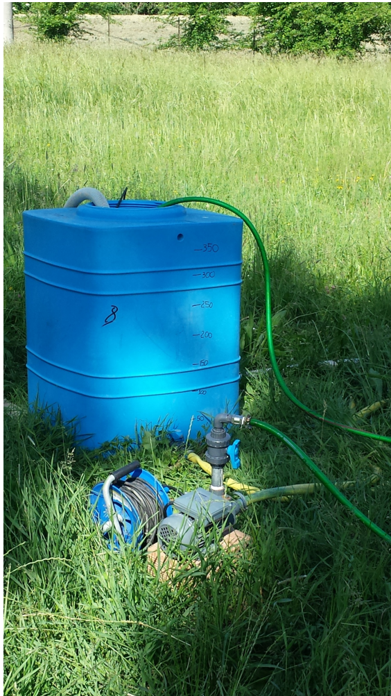
Figure 7.20: Tank used for storing the water during the oscillatory pumping tests.
