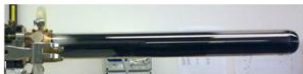
Figure 53: picture of the thermal exfoliation step. On the bottom it is possible to compare inside the quartz tube the volume of the GO precursor and the produced TEGO
