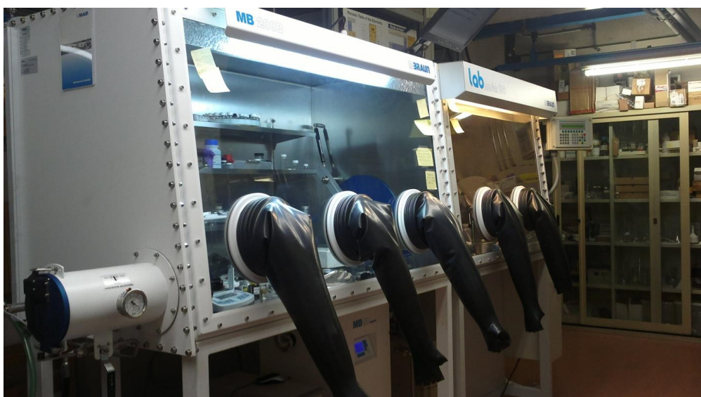
Figure 55: glove box ( \text{O}_2 and \text{H}_2\text{O} < 0,5\text{ppm} ).
