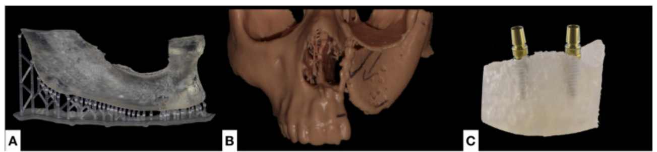
Figure 2. Examples of anatomical models fabricated by Additive manufacturing. A: A mandible model fabricated using SLA to serve as a template for bone allograft preparation during surgery. B: A model fabricated using SLA to visualize the extent of a bone defect.
