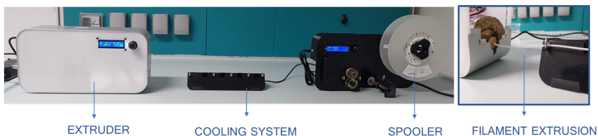
Figure 1. Extrusion system composed by a filament extruder, a cooling fan array and a spooler.
