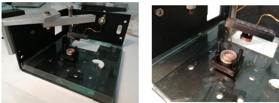
Figure 6.2-1: experiment set up for the ferroelectric measurements.
