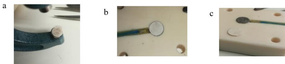
Figure 4.1.4-5: a) tablet of [\text{NH}_4][\text{Mn}(\text{HCOO})_3] after exposure at RH = 70%, b) tablet of [\text{NH}_4][\text{Mn}(\text{HCOO})_3] after exposure at RH = 90% with crystallinities on the surface c) deformation of the tablet of [\text{NH}_4][\text{Mn}(\text{HCOO})_3] after exposure at RH = 90%.
