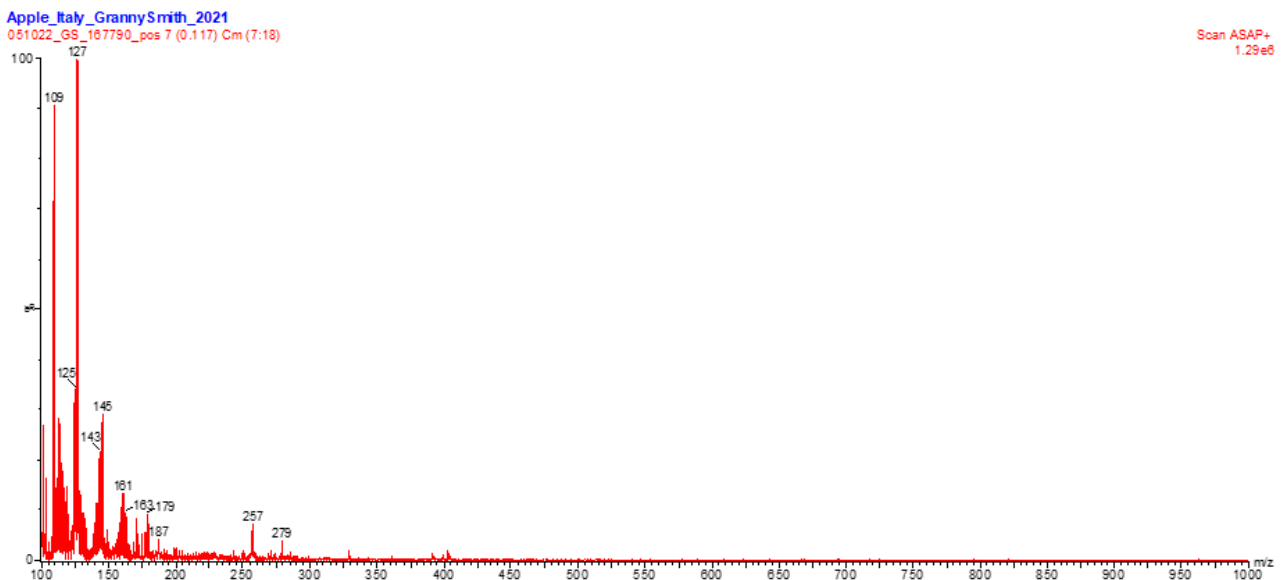
Fig. 5 ASAP-MS raw spectrum from dehydrated apple sample acquisition. Below, the background's recorded spectrum of the same sample, taken before the TIC peak.
