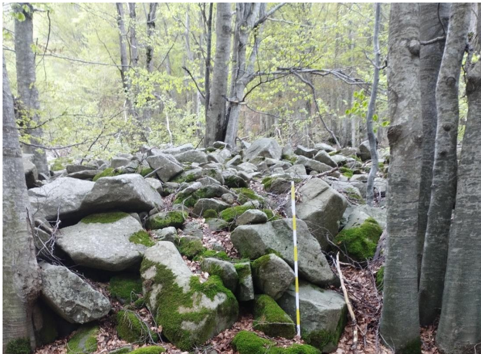
Figure 6.3: Schematic representation of debris flow body and deposits (the length of stick meter is 100 cm) (modified after Bardou, 2002).
