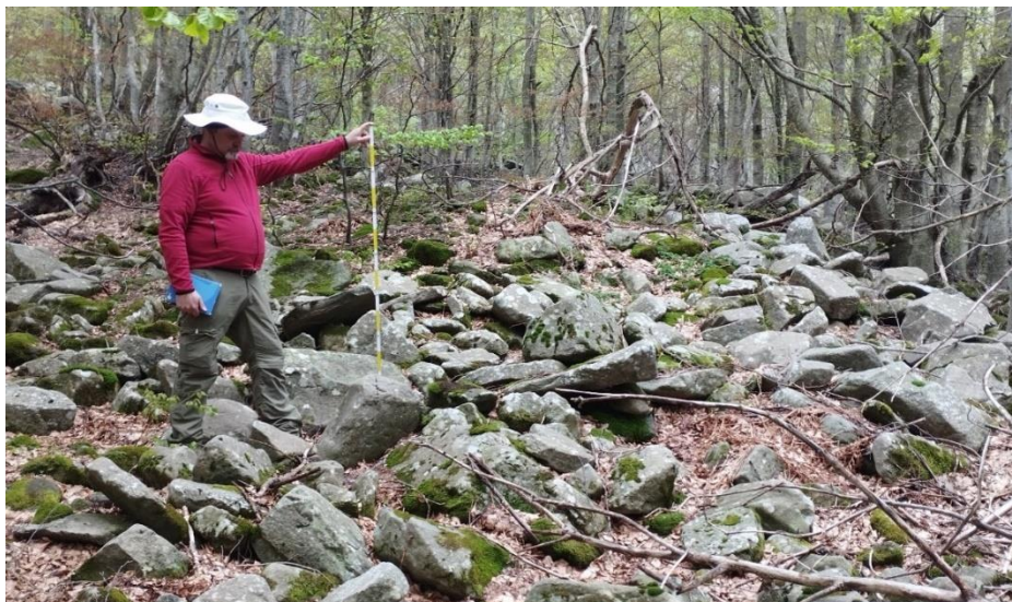
Figure 6.18: Illustration of poor sorting and lack of stratification in debris-flow deposits in channel 4 (the length of stick meter is 130 cm) (12/04/2023)
