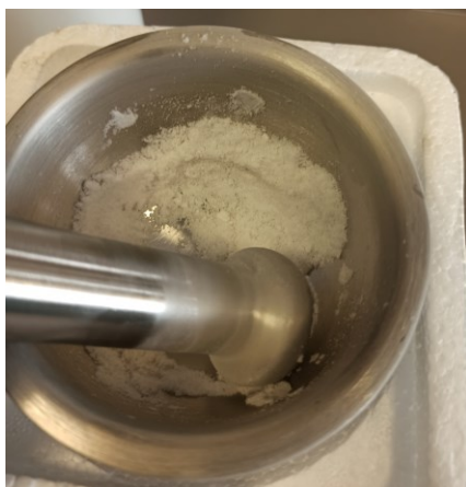
Figure 50. Stainless steel mortar (volume 250 ml; diameter 10 cm) in liquid nitrogen bath (expanded polystyrene box) containing grinded vitreous body, obtained by cryomilling.
