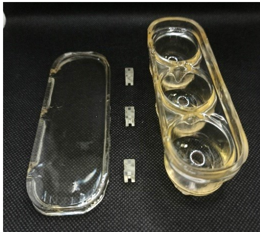
Figure 46. The final Ocutainer device, including the lid and the three tubing inserts after being coated with an epoxy resin for increased durability.
