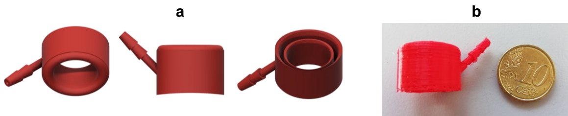
Figure 34. 3D rendering at different positions of the second version of the Ocludonor device (a) which was printed using the FDM technique in PLA filament (b).
