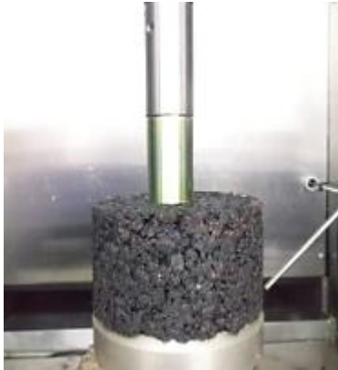
1051 1052 Figure 11. Conducting penetration shear test [87]
