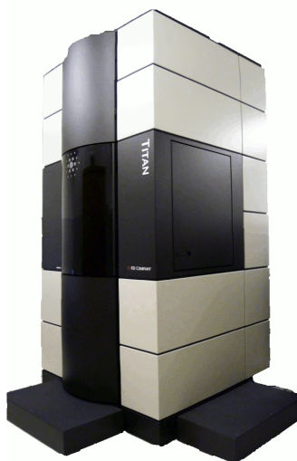
Fig. 1.25 Employed TEM microscopes, installed at IMEM-CNR (top) and LMA-INA (bottom), respectively.
