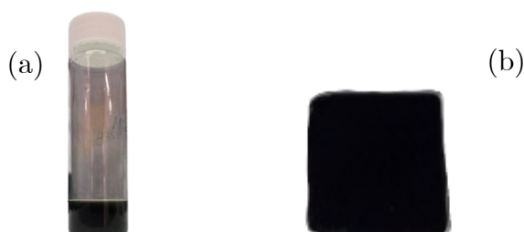
Figure 38: Picture of (a) Black Chalcogenide ink and (b) a glass slide on which the CISE ink was deposited with a brush.
