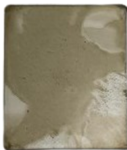
Figure 49: Picture of the CIGS dried films, deposited with spin coating method on FTO substrates of size 1\text{ cm}^2 , with the varnish stabilized in 2-propanol.
