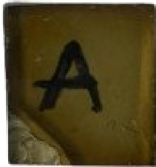
Figure 54: CIGS film deposited via Spin Coating with the centrifuged varnish. The letter “A” is written on a paper at the bottom of the sample, indicating the transparency of the film
