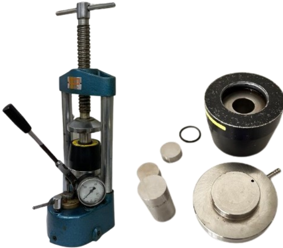
Figure 56: Experimental setup used for the cold pressing treatments on the samples. On the left, the cylindrical die inside the manual hydraulic press. On the right, the disassembled cylindrical die.
