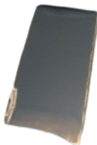
Figure 63: Picture of the film obtained with n-butanol+20%vol MEA varnish deposited via doctor blade.
