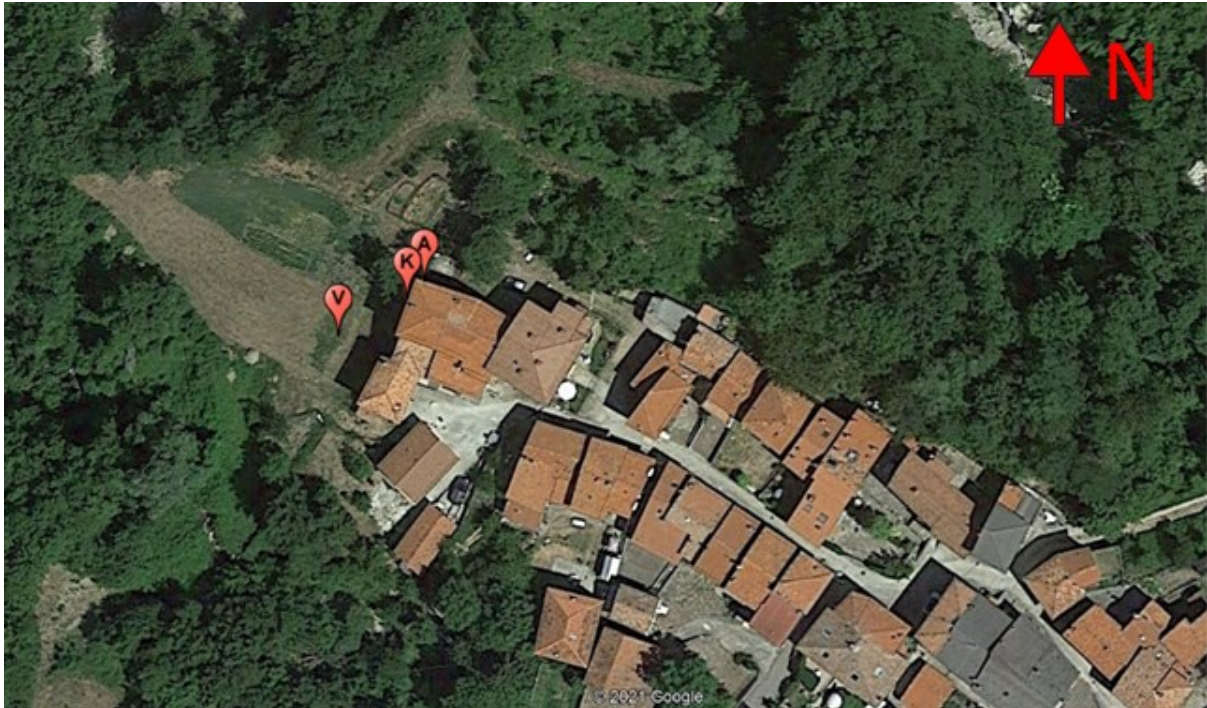
Figure 6: Measurement devices placement. V = DT0103; A = DT0003 + 1 Crack Link of DT0002; K = 1 Crack Link of DT0002. Source: (Bertolotti, 2022).
